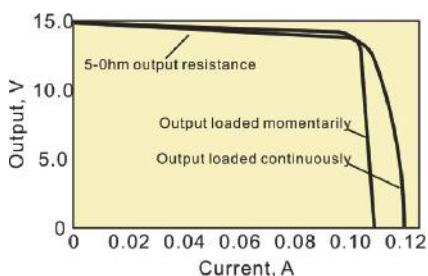
When the load exceeds the rated current (0.1A), the output voltage drops rapidly.
