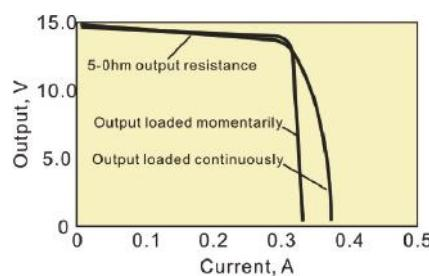
When the load exceeds the rated current (0.3A), the output voltage drops rapidly.
