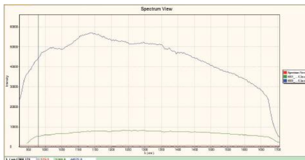
Comparison of Xenon Lamp Spectral Testing (BIM-6805 & BIM-6809)
