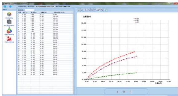
The curve showing the relationship between current and luminous flux
